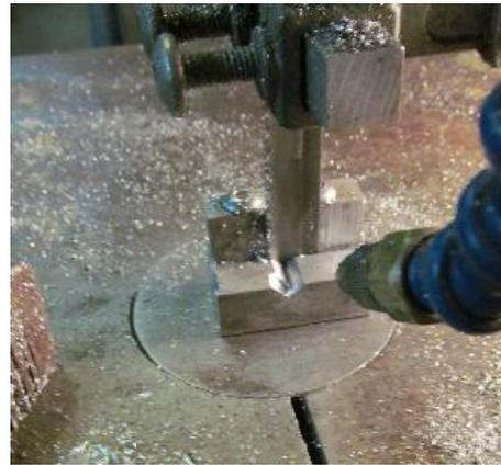
You can now measure the length of the tube/pin needed with an 'official' depth gauge or maybe a screw, a nut and a ruler. Scribe that length on the material, clamp it in the jig with the mark just to the right (see above) of the saw cut in the base, and go to the saw. Make the cut and keep a finger tip on the part to the right so you don't have to go looking under the table to see where it bounced.
