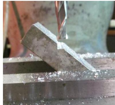
What you end up with is a bar with two “V” shaped cuts. Mark off a line at the mid point paralleling the cuts and another line at right angles to the first and about 1/3 of the way across.
