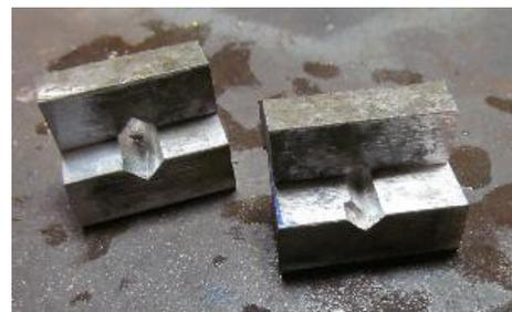
Match the blocks such that the “V”'s define a square. The one on the left is correct, the one on the right needs to be flipped over to be correct.
