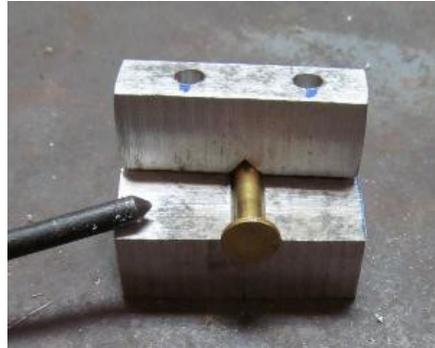
Then tap the lower block for the designated screw size. The tool shown here is a “Tap and Reamer Aligner” (Enco Model #325-4924 at ~\$75). It is also carried by MSC. It doesn't take too many broken taps before dropping the money begins to make really good sense.
